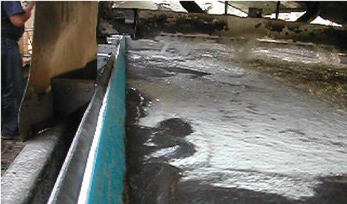
The lower part of the lateral protections, close or in contact with the drainage belt, is in rubber material. It is fixed between the stainless steel frame and the Teflon. Another rubber layer in the form of used conveyor belt has been provided over the Teflon and the cloth slides over this rubber.
