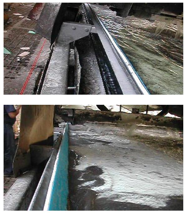
The lower part of the lateral protections, close or in contact with the drainage belt, is in rubber material. It is fixed between the stainless steel frame and the Teflon. Another rubber layer in the form of used conveyor belt has been provided over the Teflon and the cloth slides over this rubber.
