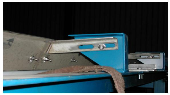
The drainage belt is not provided with the traditional two edge flanges, but it is provided for the entire length with fixed lateral protections in Teflon, supported by a frame in SS material.
